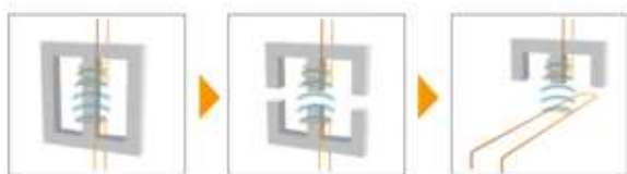
Fig. 1. Conversion from a closed conductive electric circuit to an inductive transfer of electricity (PRIMOVE I, n.d.)
